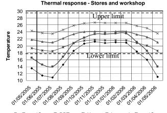
→ Ext Temp °C → TnDBT → TnUp → TnLo → Int Temp °C Figure 4: showing the thermal response of the stores and workshop to changes in exterior temperature on a month by month basis from May 2005 to May 2006.
