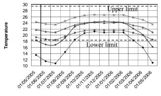
→ Ext Temp °C → TnDBT → TnUp → TnLo → Int Temp °C Figure 3: showing the thermal response of the showroom to changes in exterior temperature on a month by month basis from May 2005 to May 2006.
